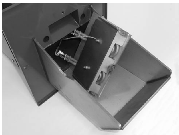
Fig. 4 - Disassembled plate with the ignition spirals
