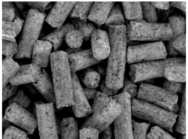
Fig. 18 – Poor-quality wooden pellets – dark with bark (with black dots)
