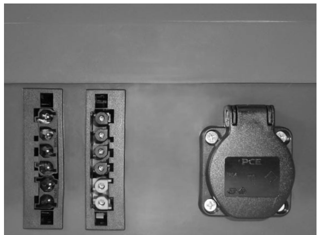
Fig. 12 - Burner with two 6-pin connectors, left - power, right - sensors and socket for conveyor
